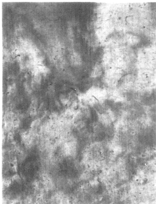
Figure 6. Polarized optical micrograph (magnification 80 \times ) of the anisotropic texture observed on cooling NBE CN and 1-6 block copolymer (89 + 50, 38/62 (w/w)) at 50 ^{\circ} C.
