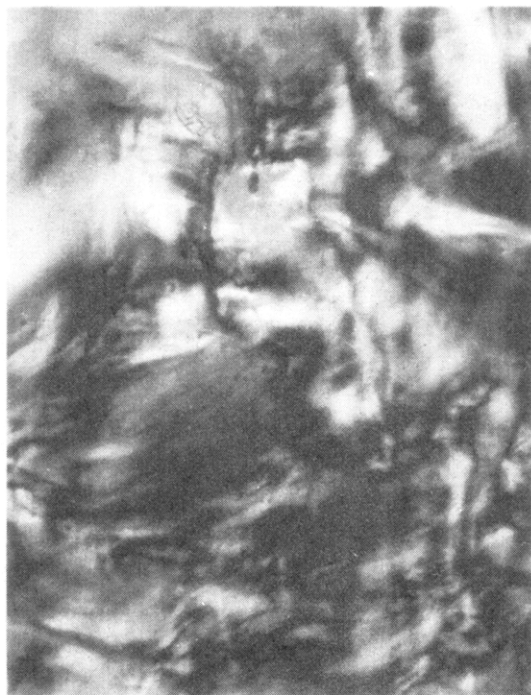
Figure 4. Polarized optical micrograph (magnification 80 \times ) of the anisotropic texture observed on cooling NBE and 1-6 block copolymer (100 + 20, 49/51 (w/w)) at 87 ^{\circ} C.
